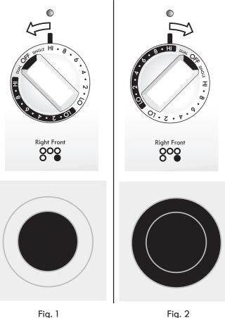
Heating with inner (small) element only Fig. 2 Heating with both elements
